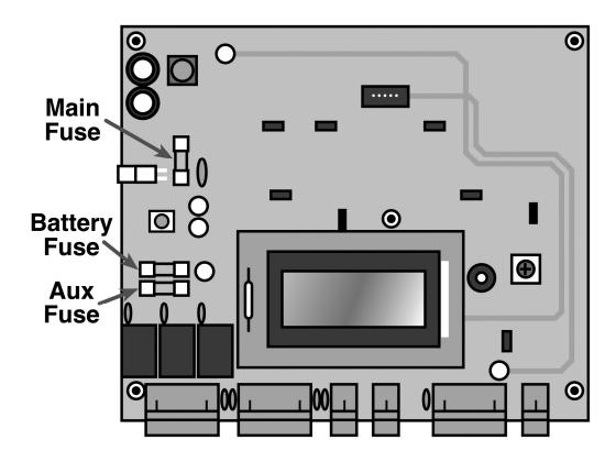
Main Fuse: Unit displays a battery symbol, and not the mains power symbol (plug).
