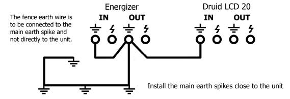
Note: Diagrams illustrate connections of only 1 zone for simplicity. Both zones can be wired as shown.
