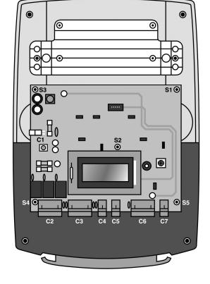
**STEP 5:** To replace the PC Board, align the four spade connectors in the middle of the PC Board using the guide tabs, and gently press the PCB down into place.
